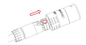
(6) After the assembly of the cable clamp, inner core and housing, tighten the boot in a clockwise direction.
