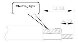
(3) Solder the conductor of the cable to the inner core assembly and secure the cable with the clamping plate.
